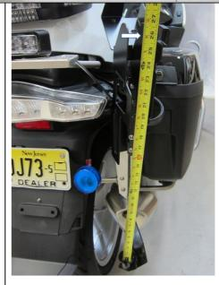
Secure the top two M6 x 20 Torx bolts and M6 nylock nuts.
