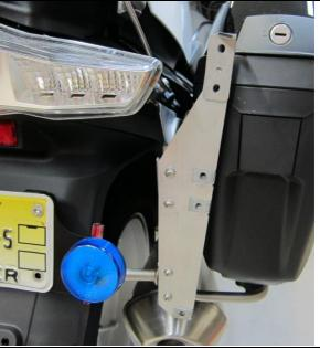
Secure the upper assault rifle mount to the upper two holes in the bracket using the M6 x 16 Torx bolts, securing with M6 nylock nuts. Snug but don't tighten fully yet.
