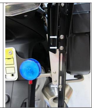
Earlier production rifle mounts are drilled and tapped for an M5 x .8 threaded pin to provide a more convenient pin location for the retaining strap – included with Long Rifle mounting bracket orders. Later production simply moved the pin to the noted location for all mount types.
